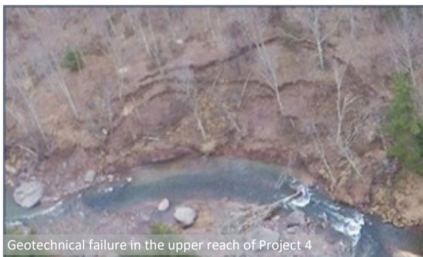
Lateral migration, down cutting, and toe erosion causing upgradient failures.
