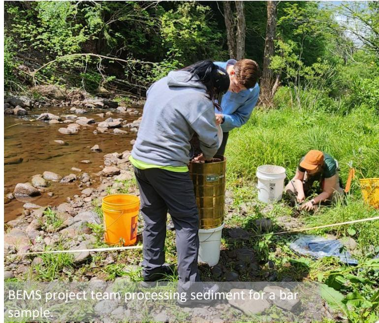
BEMS project team processing sediment for a bar sample.
