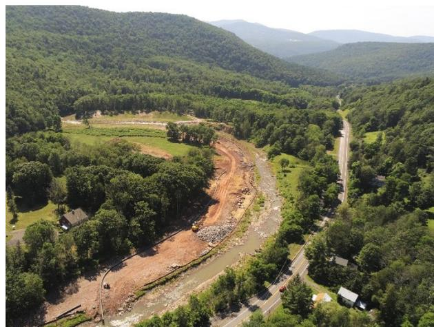
This current condition of the reach increases the risk for potential hillslope failure and impact on the highway and private bridge foundations, thus reducing public safety. The existing incised clay-lined channel is causing water quality degradation of the drinking water supply and significant trout habitat impairment due to nearly continuous turbidity.
