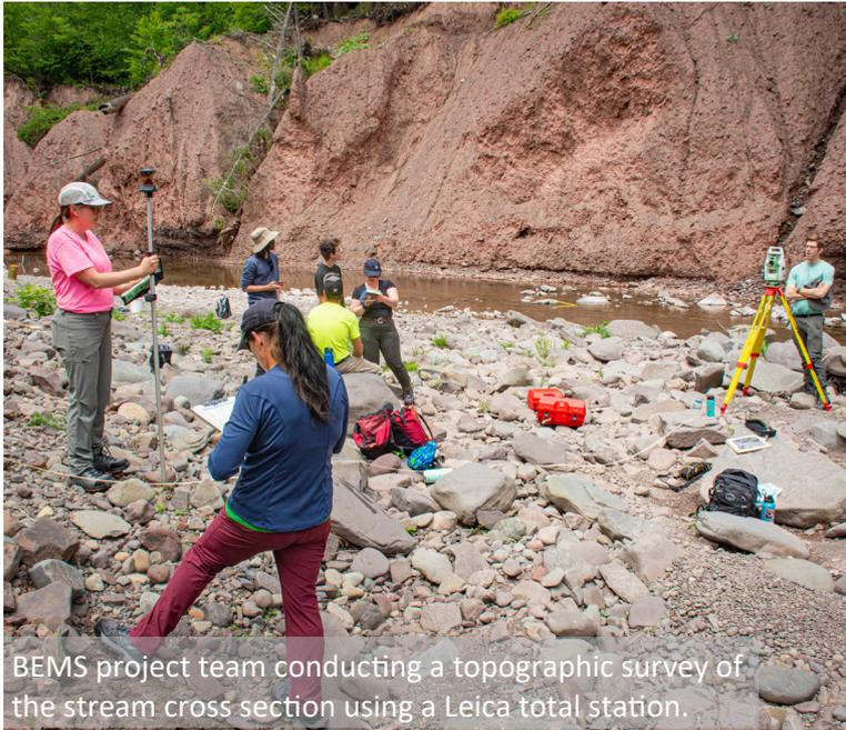
BEMS project team conducting a topographic survey of the stream cross section using a Leica total station.
